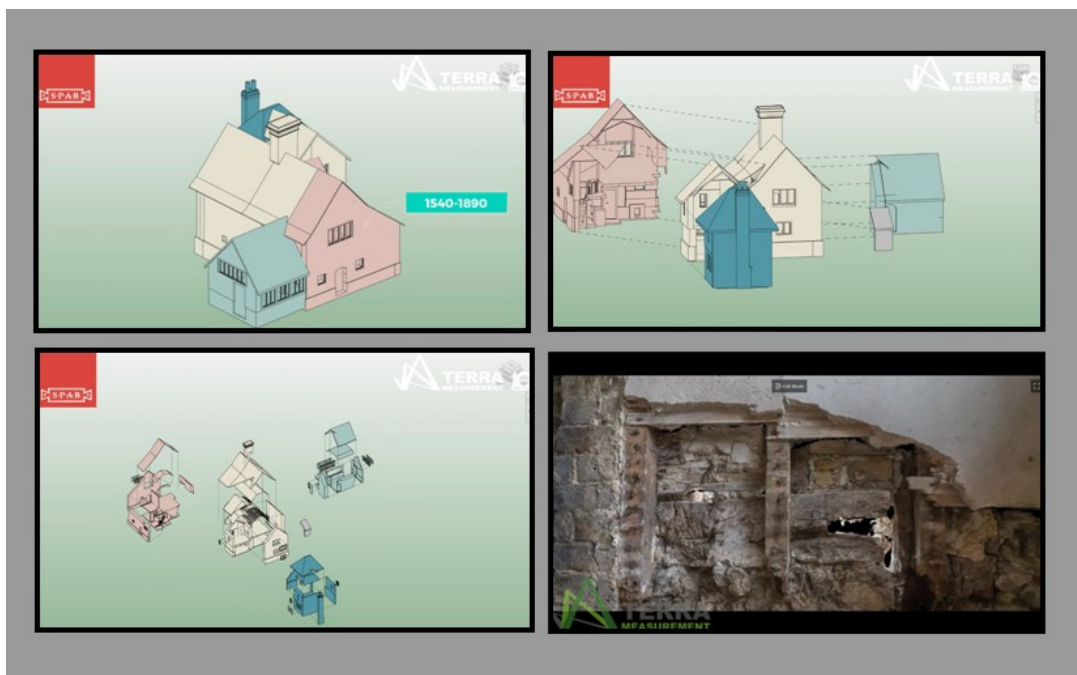
Fig.6. 3-D laser visuals to aid understanding of phases and building details ©Terra Measurements reproduced courtesy of SPAB.
