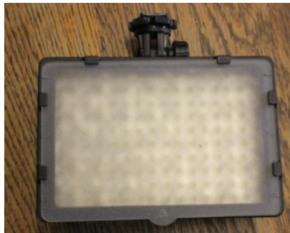
Fig.1. On camera, continuous halogen light unit which slots into the 'hot shoe' on top of the camera.
