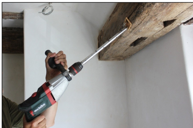
Fig.3. Dr. Martin Bridge from the Oxford Dendrochronology Laboratory extracting a core.
