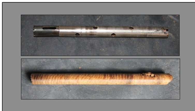
Fig.1. Drill core bit and resulting timber core.
