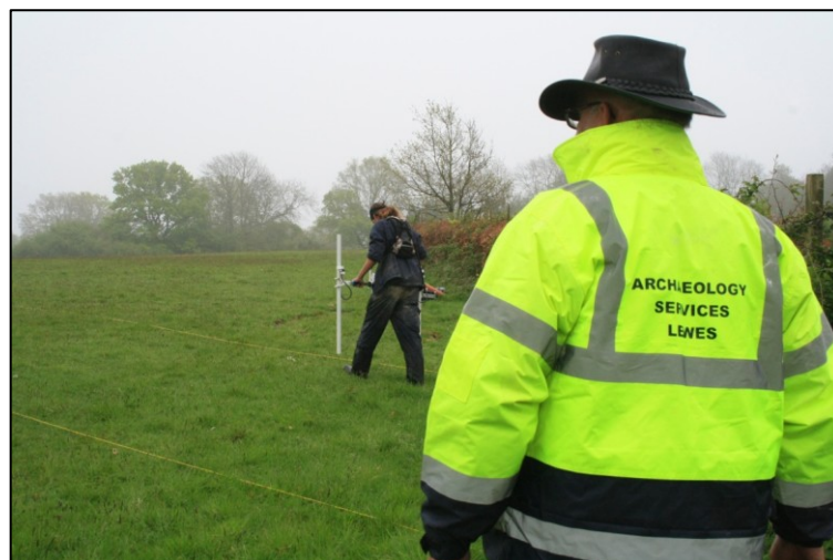
Fig.5. Magnetometer survey walked in grid lines.
